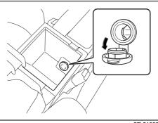
The accessory socket will work when the ignition mode is changed to "ACC" or "ON" by pressing the engine switch.
